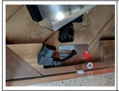
Unplug the heater cord from the floor cord and remove the heater.
